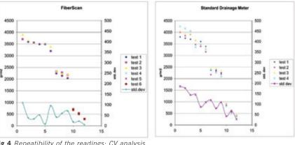
Fig 4 Repeatibility of the readings: CV analysis
