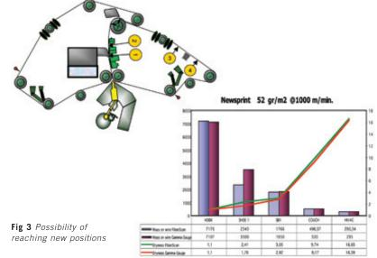
comparison between FiberScan™ microwave meter and the standard
